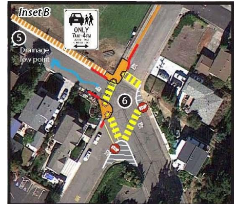
Proposed changes to this intersection at Robert Semple include upgraded curb ramps, high visibility crosswalks, and low-cost striping near the tunnel entrance under I-780
