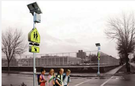
Rectangular Rapid Flash Beacons (RRFB) increase yield compliance at uncontrolled crossings.
